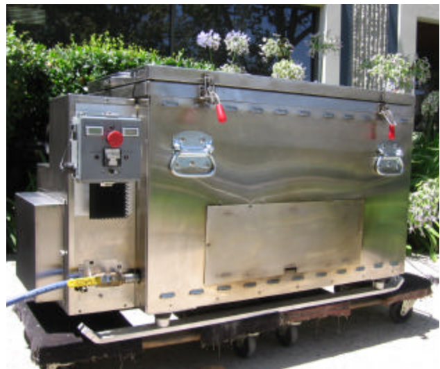
Figure 8. Self-powered tray ration heater
