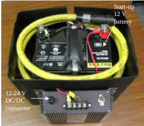
Figure 13. STRH Battery Pack
