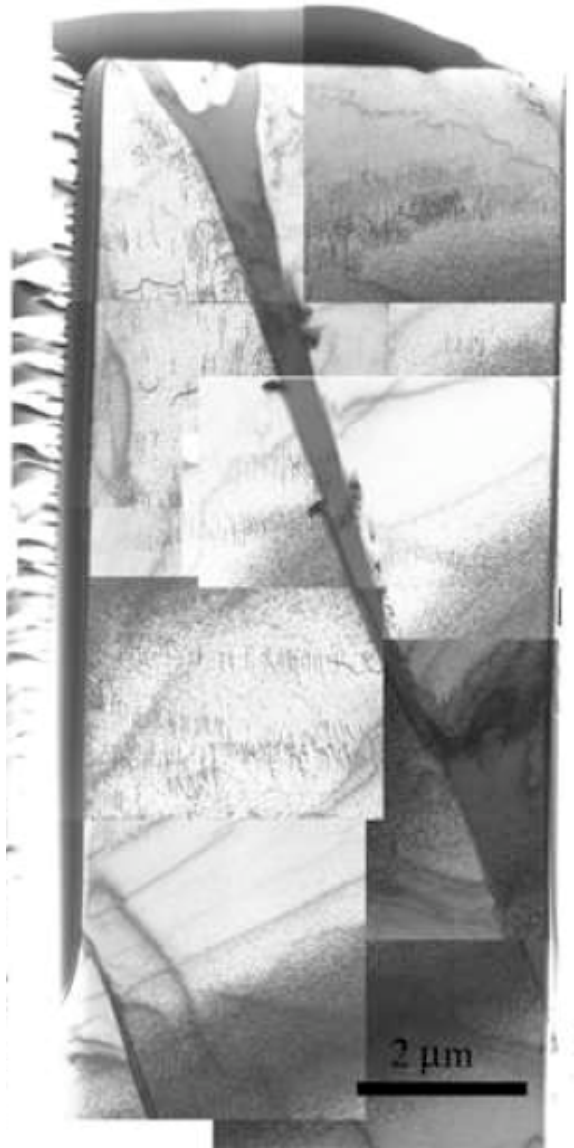
Figure 16. BF-TEM images taken from a 5 \mu\text{m} Ti-6242 longitudinal foil, such that the Burgers vector is out of the plane of the foil.
