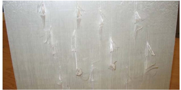
Fig. 3. An MBPS panel after RCC testing
