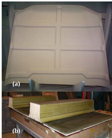
Fig. 6: (a) M35A3 hood and (b) hat stiffened structure for Advanced Sail Program and DDX prepared using FAVE-L resin.
