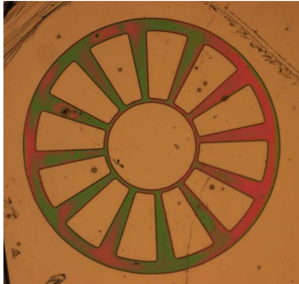
Figure 6-5: Photoresist pattern on HOPG thin film application to PolyMUMPs ® die.
