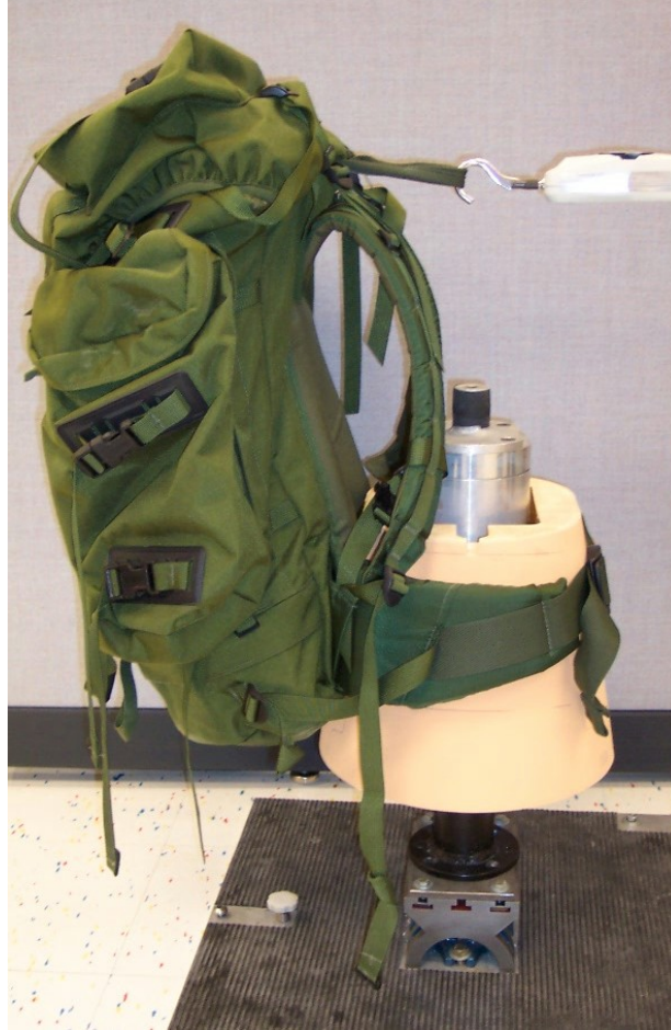
Figure 10. Pack placement for isolated waist belt testing.
