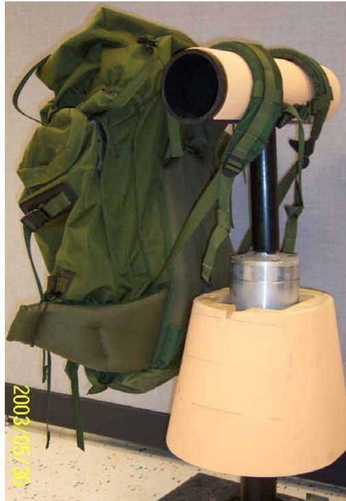
Figure 12. Pack placement for isolated shoulder testing.
