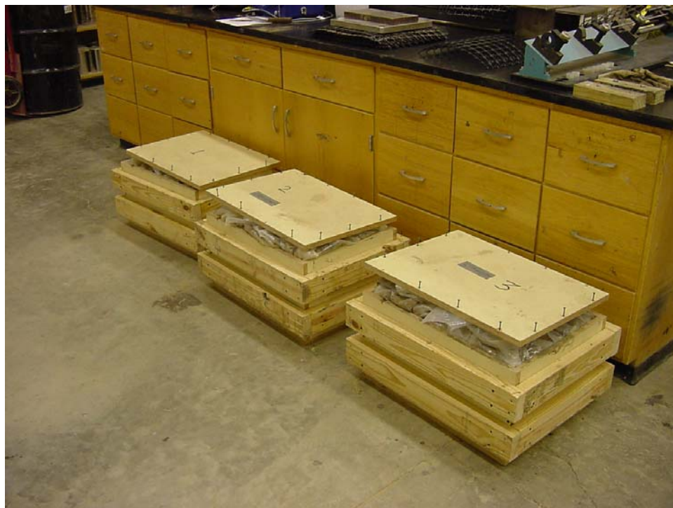
Photo 9. Wet soils are sealed for the equilibration period.
