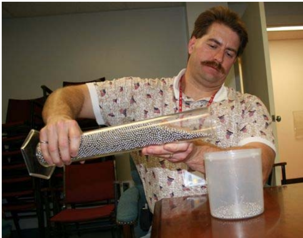
Photo 19. Pouring balls from graduated cylinder into beaker with known volume.
