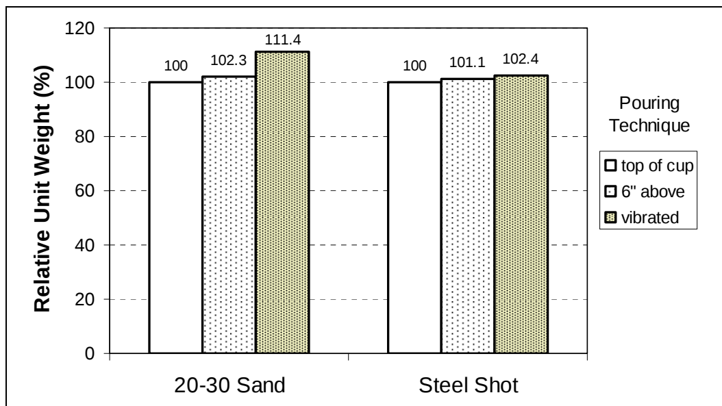
Figure 2. Relative final unit weights for different filling procedures.
