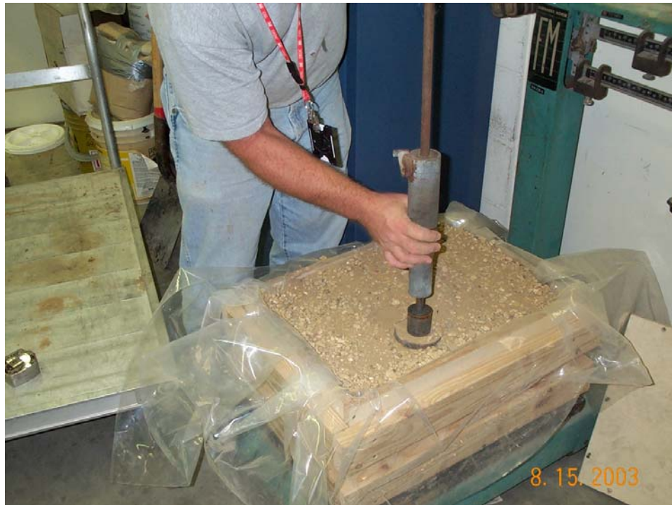
Photo 8. Compacting soil for the moisture content tests.
