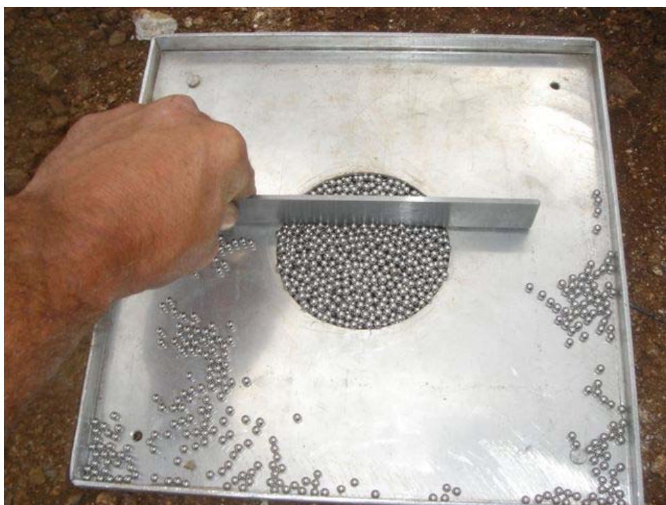
Photo 30. Striking off excess steel shot.
