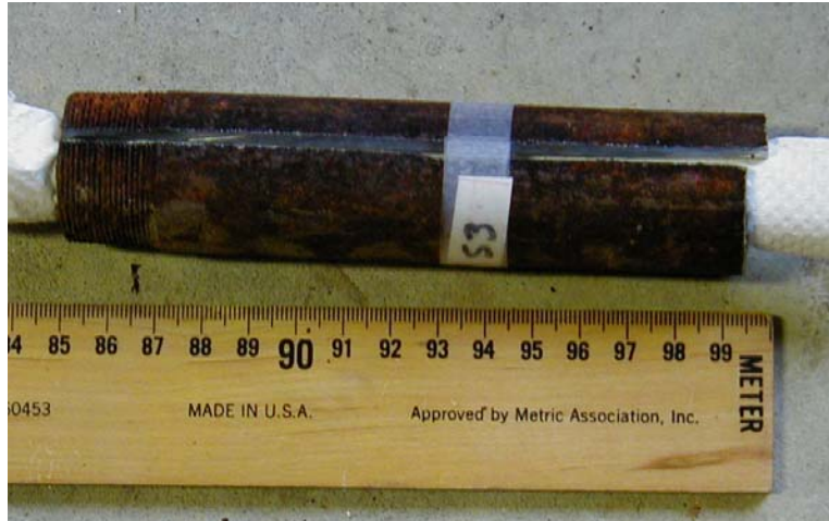
Figure 65. Section of steel pipe with longitudinal cut.
