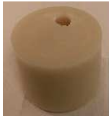
Fig. 3. Photograph for gelatin phantom (representing the idealized two-dimensional cross-sectional geometry shown as first column in Fig. 4(a)) used in the experimental studies.
