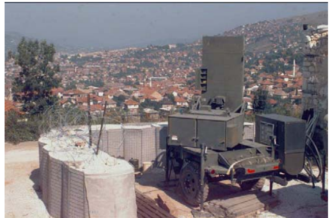
Fig. 1. A Fire Finder radar system that could operate more efficiently and have a wider bandwidth if GaN HEMTs were substituted for GaAs HEMTs.
