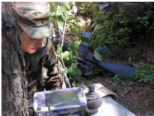
Figure 3 A dismounted Soldier uses the SUGV OCU
