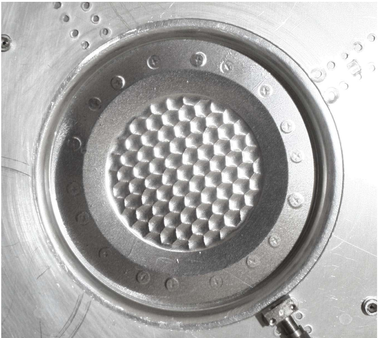
Figure 6. Initial atmospheric loading of 12.7- \mu m thick 1145/12355-H19 aluminum foil.
