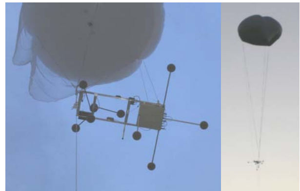
Figure 4. Two array systems for transient localization on 25' diameter balloon, relative position of array hanging from balloon.
