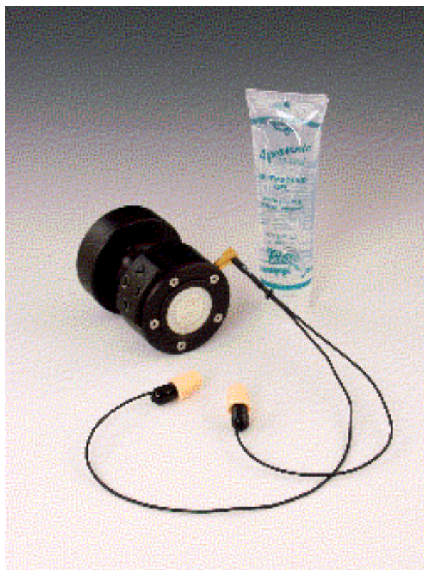
Figure 3. Stethoscope connected to Communications Earplugs® (made by Communications & Ear Protection, Inc.), and gel used for ultrasound mode..
