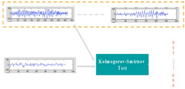
Figure 10: System architecture of buried mine classifier.
