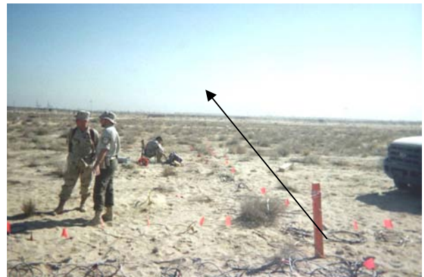
Figure 7. Surface layout of the data collection array. Tunnel direction is in direction of tunnel
