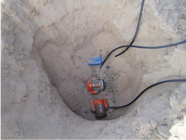
Figure 4a. Geophones used in the study.
