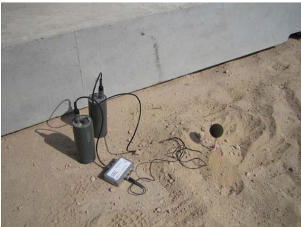
Figure 5b. Acoustic sensor with windscreen.
