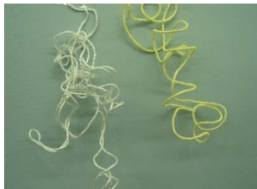
Fig. 8 OPH-PTH cotton thread recovered before (left) and after (right) MPT degradation
