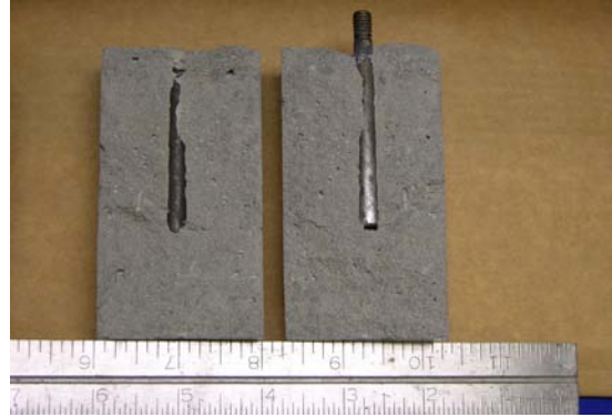
Fig. 2. Mortar cylinder split after testing to show the surface of the glass adhering to the hardened mortar and the clean surface of the metal test rod. Examination of the surface of the glass showed fragments of metal embedded in the glass.
