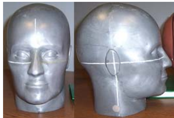
FIGURE 4: The USAARL headform models the average US Army soldier facial anthropometry.
