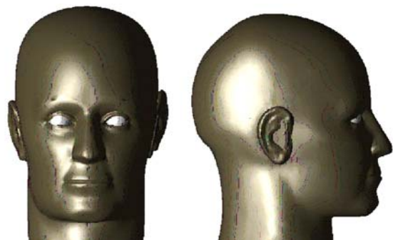
FIGURE 5: The FOCUS headform exterior geometry is modeled after the specified USAARL headform.
