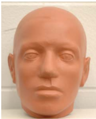
FIGURE 3: The ANSI headform has the correct anthropometric features for testing eye and face protection, but no instrumentation for measuring impact forces.
