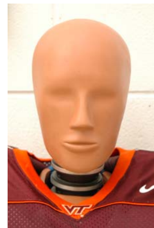
FIGURE 2: The Hybrid-III headform lacks detailed facial features.
