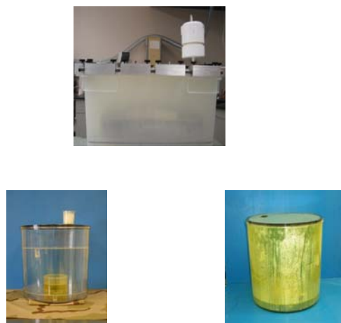
Figure 6. Two early versions of the PCS. Top: 32-gallon tote with homemade filter unit. Bottom a 1 ft 3 plastic bucket (left) before and (right) after initiating the chemical production of \text{ClO}_2 .
