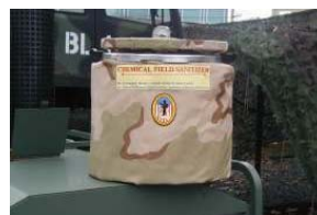
Figure 4. Original PCS prototype was an insulated COTS pressure cooker and MRE heaters in water to effect sterilization through the production of “wet heat” (temperature above 121 °C and copious steam).
