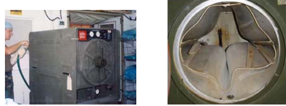
Figure 2. (Left) large “Bertha” steam autoclave at CSHs; (Right) collapsed inner chamber of “Bertha” due to overuse and limited maintenance capabilities.
