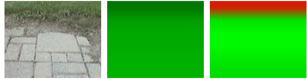
Fig 7: Measured vehicle-terrain interaction parameters ( \alpha = center and \rho = right).
