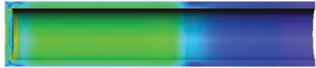
Figure 12. Von Mises stress in the projectile at 4.8 ms into the shell-loading simulation. The peak stress at this time is 705 MPa and occurs at the center of the rear face of the projectile.
