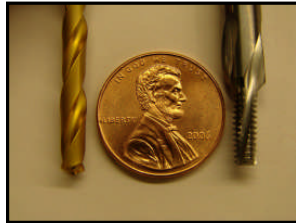
Drill and #10-32 Threadmill
