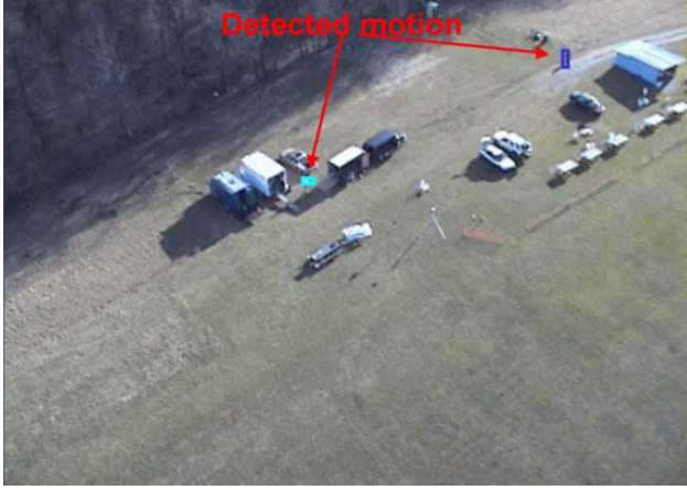
Figure 3: Sample frame from a video sequence recorded with the CMU helicopter, showing the detection of the two moving persons.
