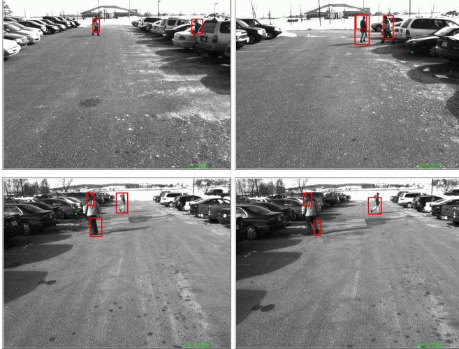
Figure 8: Sample detection results for ground level MTI. The red boxes denote image areas where independent motion was detected.
