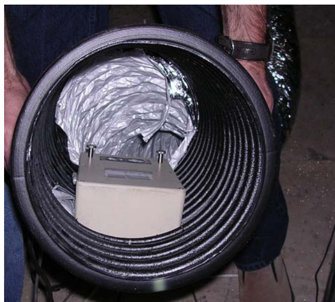
Figure 5. RAS installed in plastic drain pipe and mounted at end of model gopher tortoise burrow.
