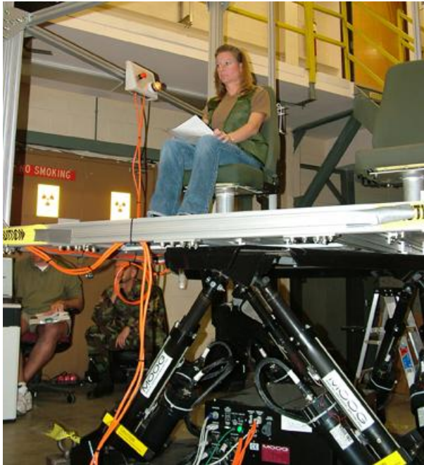
Figure 3. A six-degree-of-freedom Ride Motion Simulator (RMS) was used to simulate movement of a High Mobility Multipurpose Wheeled Vehicle (HMMWV) and a Bradley Fighting Vehicle (BFV) moving over gravel and cross country terrain at an average speed of 20 mph.
