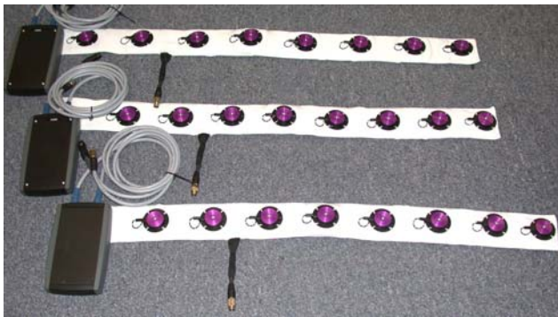
Figure 2. Three tactile displays belt assemblies are shown above along with their Tactor Controller Boxes (TCB). Each box includes a wireless Bluetooth receiver and the controller circuitry and waveform generator.
