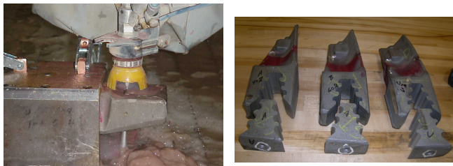
Water jet cutting techniques being tested (left). Water jet cut parts at three different parameter sets (right).
