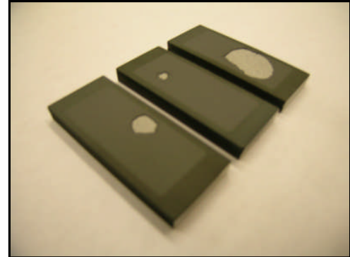
Figure #14 Saint-Gobain Coating Solutions Rokide-C Chrome Oxide STG-A-R1, R2, R3 Rain Erosion Test
