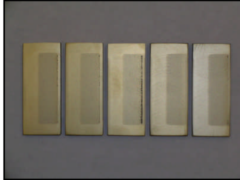
Figure #15 MDS-PRAD Technologies Corporation Titanium ER-7 TiN MDS-P1, P2, P3, P4, P5 Particle Erosion Test
