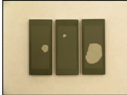
Figure #13 Saint-Gobain Coating Solutions Rokide-C Chrome Oxide STG-A-R1, R2, R3 Rain Erosion Test
