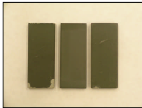
Figure #9 Saint-Gobain Coating Solutions Rokide-C Chrome Oxide STG-A-P1, P2, P3 Particle Erosion Test
