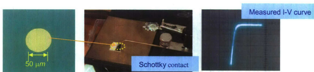
Figure 14. Fabricated Schottky diode mixers for mixing the RF signals.
