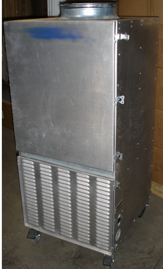
Figure #1 Typical Portable Ventilator with Air Filtration
