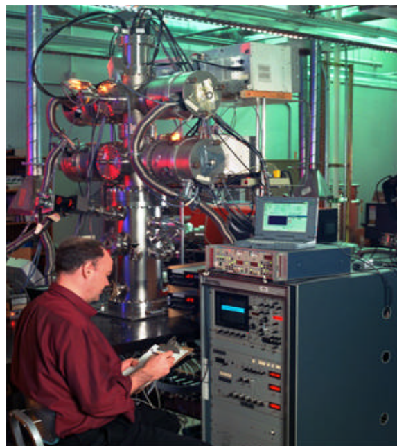
Figure 1. A photograph of our experimental apparatus. Apparatus consists of a low pressure burner equipped for MB-MS, LIF, and thin-wire thermometry.
