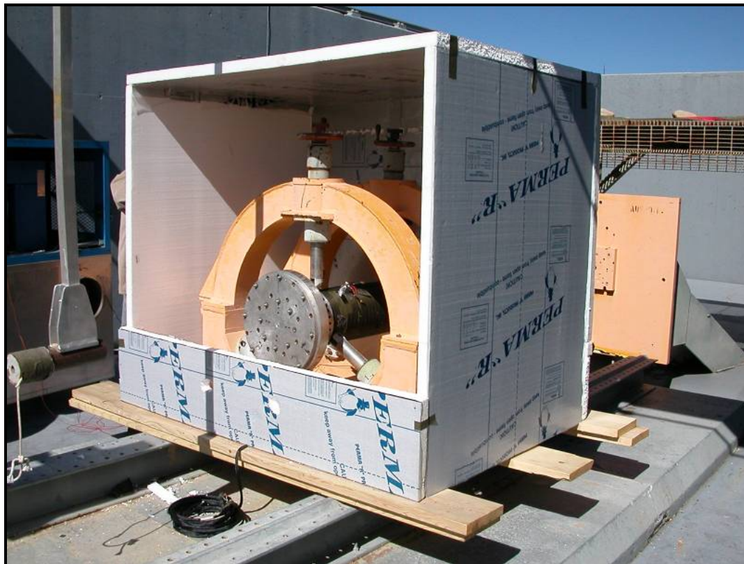
Figure 1. Open Temperature Conditioning Shroud Encompassing Entire Pyroshock System
