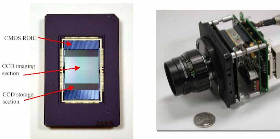
Figure 9: Prototype CCD/CMOS hybrid FPA and low level light camera (Liu et al, 2005)
