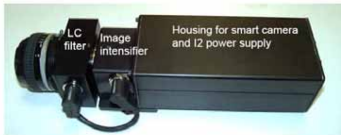
Figure 11: True-color night vision camera (ICMOS camera with Liquid Crystal Filter) (from http://www.techexpo.com/WWW/opto-knowledge )
