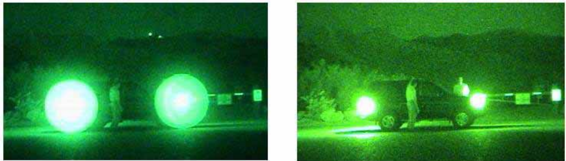
Figure 40: Comparison of anti-blooming or halo free feature (Estrera et al, 2003)
