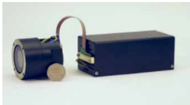
Figure 4: Micro ICCD camera system from Defence Vision Systems (from http://213.210.6.54/dvsmil/PDF )
