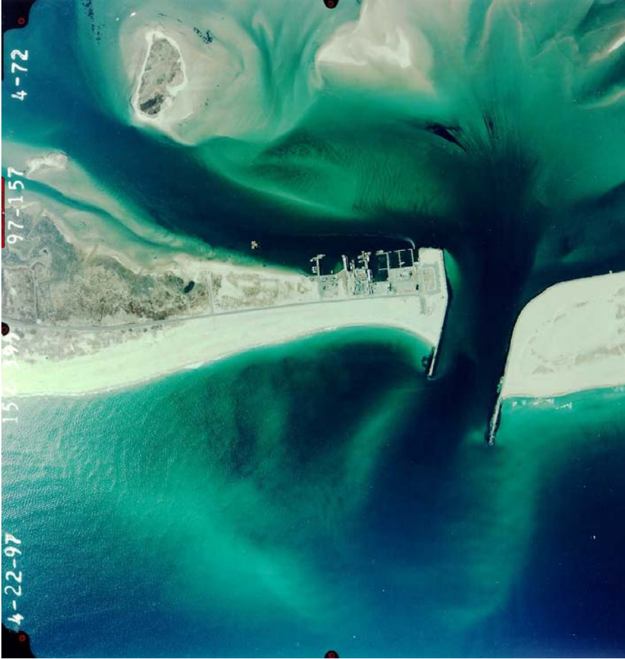
Figure 3. Aerial view of shoals at Shinnecock Inlet during a calm day, April 27, 1997. Note the shoal inside the inlet adjacent to the west (left) jetty on the bay end. Presence of this shoal is essential for creation of Threes.
