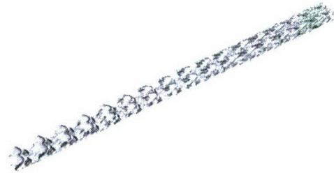
Figure 7.35: Fundamental breakdown. Vortical structures identified by the Q-criterion ( Q = 500 ). Ma = 7.95 , Re = 3,333,333 , T_\infty = 53.35K , F = 9.8 \cdot 10^{-5} , A_{1,0} = 1\% , A_{1,1} = 0.001\% , \Psi_{1,1} = 60^\circ .
