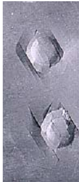
Tantalum on Gun Steel via Cylindrical Magnetron Sputtering
