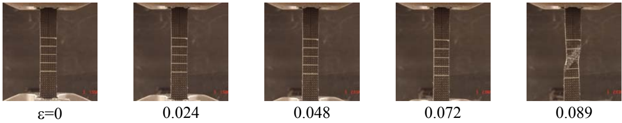
Figure 4.2-9(b) Optical pictures of a \pm 45 plain-weave woven composite symmetric GR-GL-GL-GR specimen taken during tensile testing at different strain levels.
