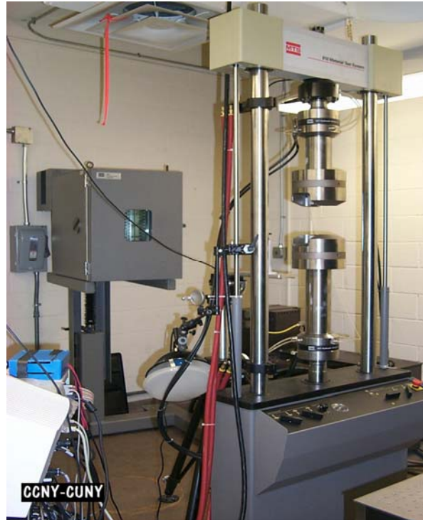
Figure 4.2-1. The MTS machine with an environmental chamber.
