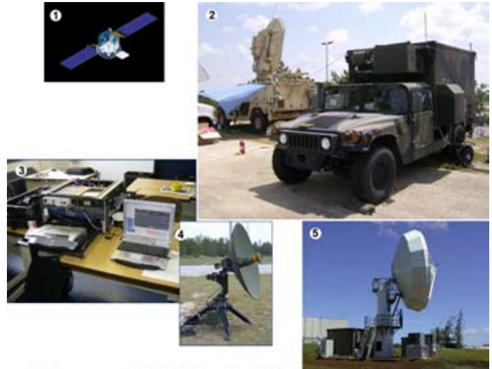
1 - Space segment: UFO satellite hosting the GBS payload 2 - Transmit Segment in Theater; Theater Satellite Broadcast Manager (truck) and Theater Injection Point (antenna) 3 - Receive Broadcast Manager 4 - Receive Terminal 5 - Transmit Segment: Primary Injection Point (white dish antenna) and Satellite Broadcast Manager (buildings)
