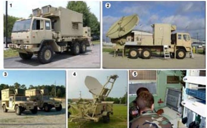
1 - Increment 1 Unit Hub Node 2 - Increment 1 Satellite Transport Terminal 3 - Increment 1 Joint Network Nodes 4 - Increment 1 Ku Satellite Trailer 5 - Operations in Shelter
