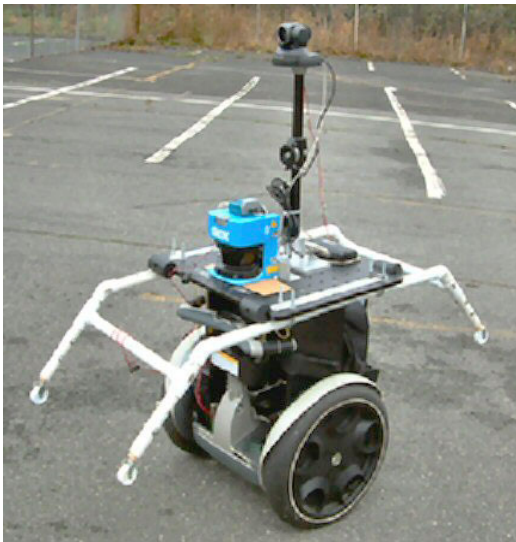
Figure 12. UMass RMP with safety system.
