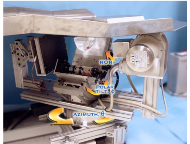
FIGURE 2. Photograph of the prototype dual-modality dedicated breast imaging tomographic system with a customized patient bed. The SPECT system (center) is placed orthogonally to the CmT tube (right) and digital flat-panel detector (left). The superimposed arrows illustrate system motions (polar and ROR for SPECT, and azimuthal for SPECT and CmT). Note that the pendant breast is in the common FOV of each system.
