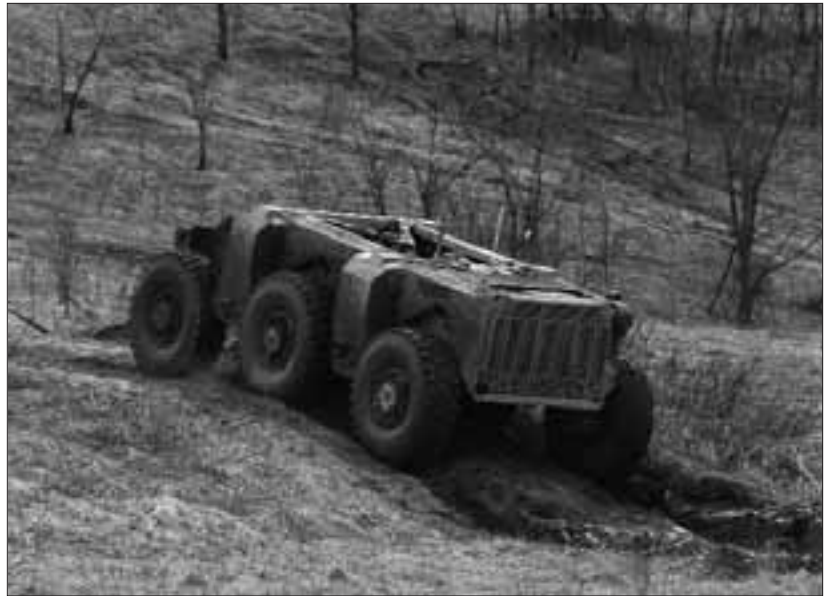
The Crusher unmanned ground combat vehicle was unveiled in April 2006 by the Defense Advanced Research Projects Agency.
