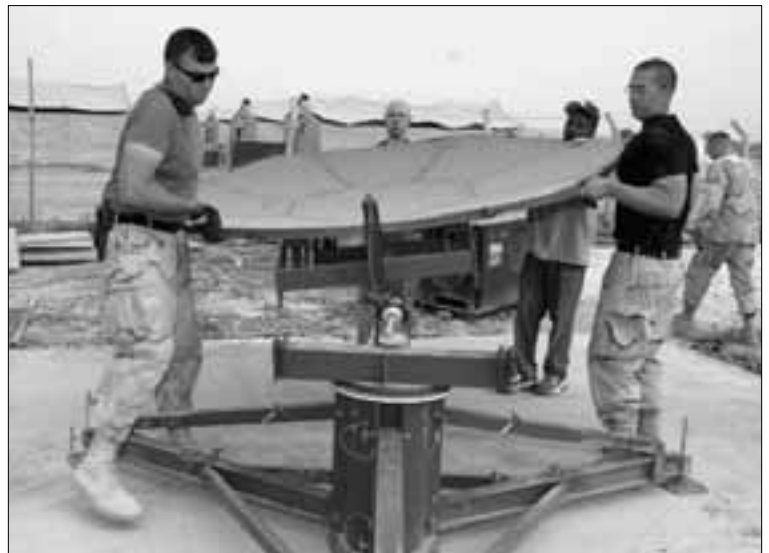
Members of the 407 Expeditionary Communications Squadron put together a Flyaway KU Band Earth Terminal (FKET) Satellite System. The 407 ECS is deployed to Tallil Air Base, Iraq.
