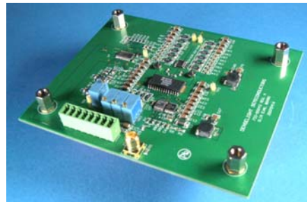
Figure 2b. Evaluation board top side where most of the electronic components are mounted
