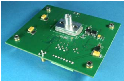
Figure 2a. Evaluation board bottom-side where the TO-8 TOSA SWIR light source is mounted
