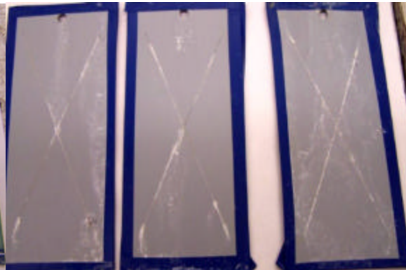
Figure 120: AC-131 + Mil-PRF+85582 (N) + Mil-PRF-85285 on Al 2024-T3 2000 hours of exposure
