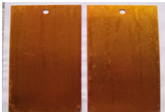
Figure 94: BAM-PPV Coated Al 2024-T3 Thickness > 1.0 micron Time = 336 hours
