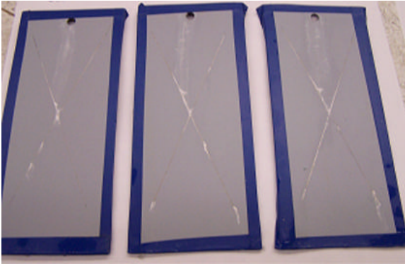
Figure 111: BAM-PPV + Mil-P-53022 + + Mil-PRF-85285 on Al 2024-T3 2000 hours of exposure
