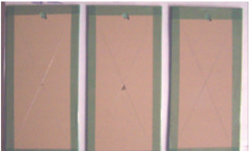
Figure 135: 1008 Steel with BAM-PPV + Mil-P-53030 + Mil-C-53039 before exposure
