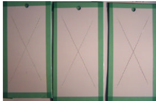
Figure 138: Powder coat with BAM-PPV on Al 2024-T3 before exposure
