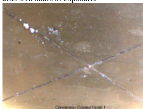
Figure 72: Scribed conversion-coated Al panel after 616 hours of exposure.
