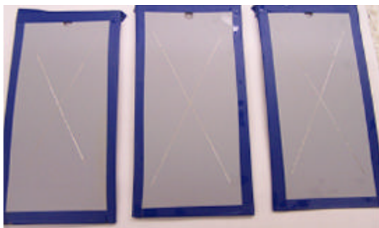
Figure 122: BAM-PPV + Mil-PRF-23377 + Mil-PRF-85285 on Al 2024-T3 2000 hours of exposure
