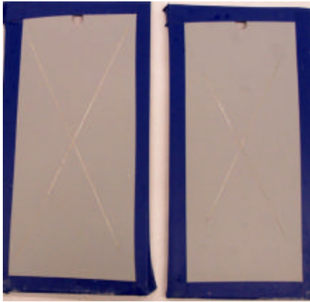
Figure 124: BAM-PPV + Mil-PRF-23377 + Mil-PRF-85285 on Al 2024-T3 4000 hours of exposure
