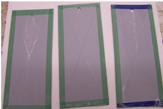
Figure 119: Alodine 5700 + Mil-PRF-85582 (N) + Mil PRF-85285 on Al 2024-T3 2000 hours of exposure
