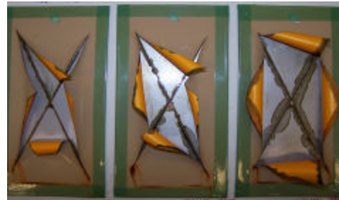
Figure 136: 1008 Steel with BAM-PPV Mil- P-53030 + Mil-C-53039 48 hours of exposure
