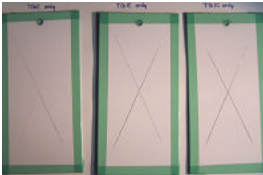
Figure 137: Powder coat control (no BAM-PPV) on Al 2024-T3 before exposure
