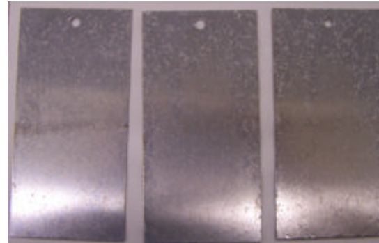
Figure 98: Alodine 5700 Pretreatment on Al 2024-T3, Time = 24 hours
