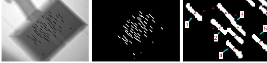
Fig. 2. (Left) X-ray image on phantom data; (Middle) the seed-only image resulted after preprocessing; (Right) Example of seed region labeling and seed grouping.
