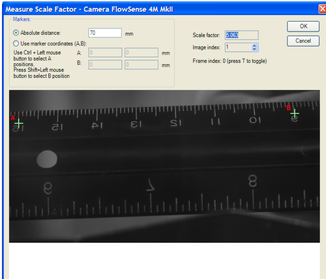
Figure 19: Calibration image with measured scale factor.
