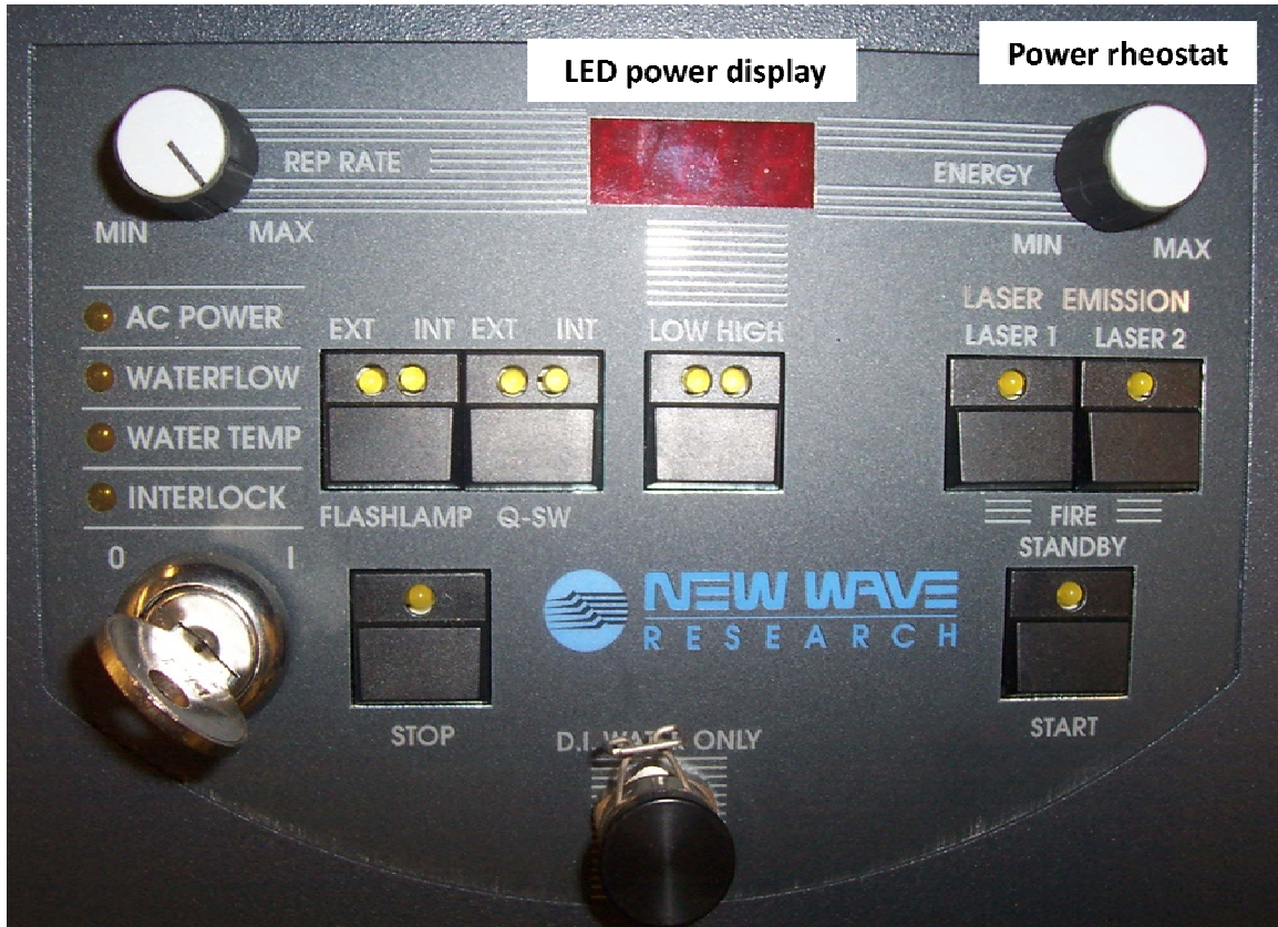
Figure 14: Control panel for Solo 200 laser system.
