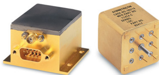
Figure 3. Model 9700 series crystal oscillator (courtesy of Symmetricom).
