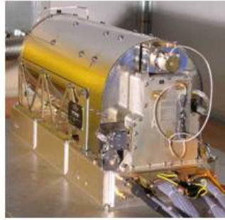
Figure 16. Hydrogen maser clock for Galileo GIOVE-B (courtesy of SpectraTime).
