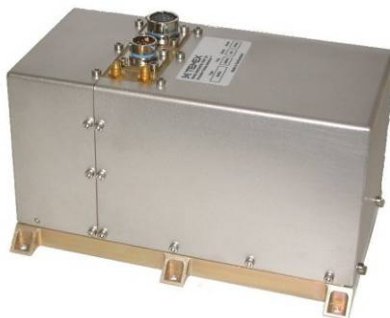
Figure 10. Rubidium clock for Galileo (courtesy of SpectraTime).
