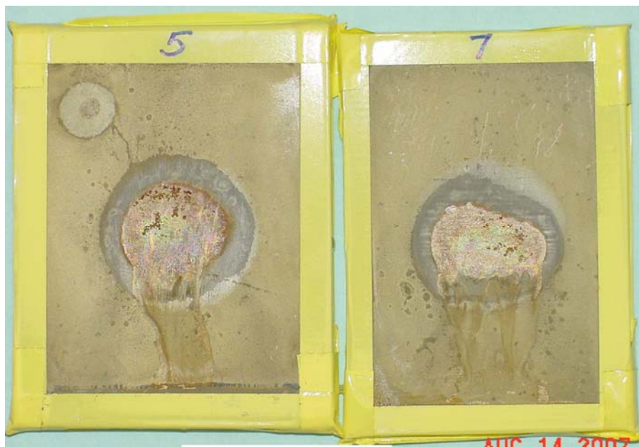
Figure 4-8 – Wafer #5 Spot Side and #7 No Spot Side at 23 hours SO 2 Salt Spray I
