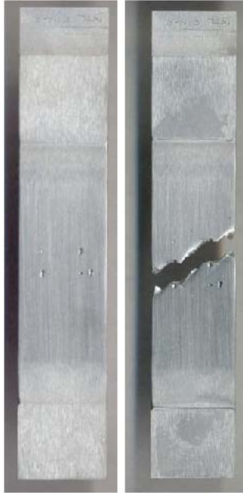
Figure 33: Pre- and post-fracture top view of specimen 598-5
