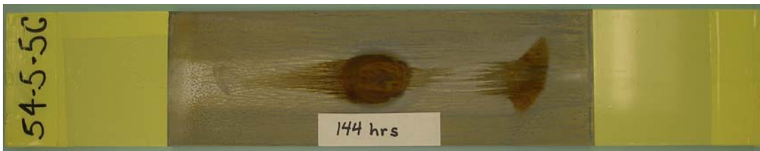
Figure 4-14 –Fatigue Bar 545-5C Corrosion at 144 Hours
