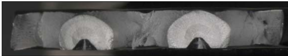
Figure 32: Fracture surface for micro-machined specimen 598-5
