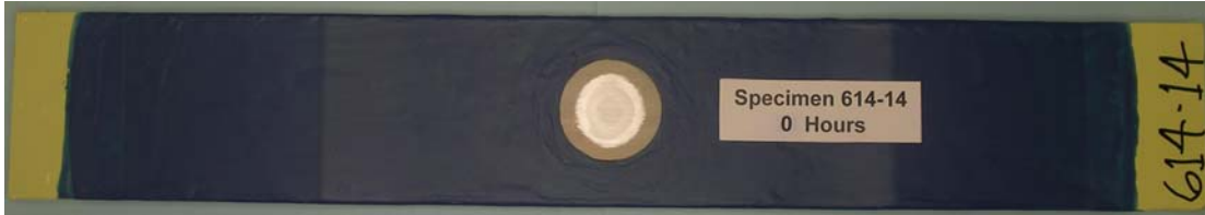
Figure 4-15 - Fatigue Bar 614-14 showing typical application of Chem Mill Maskant
