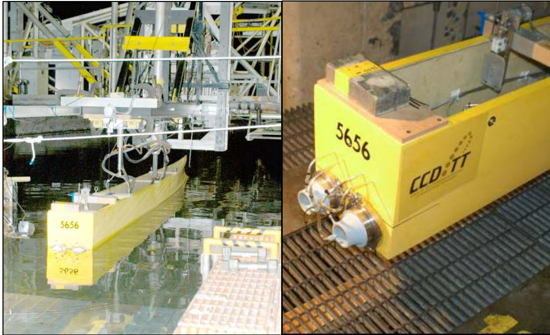
FIGURE 2 - MODEL HULL WITH WATERJETS ON THE DTMB TOWING CARRIAGE
